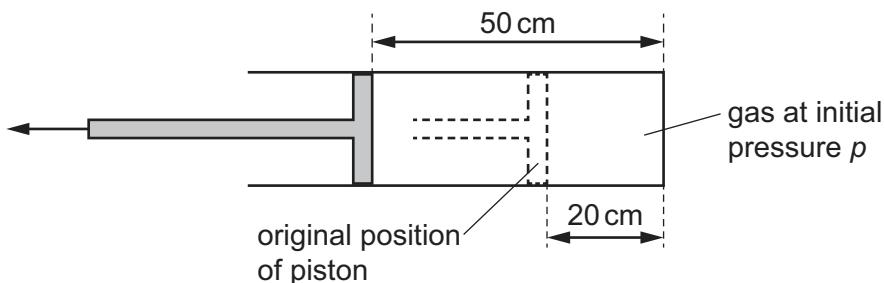
The piston is pulled out a distance of 30 cm, so that the length of the gas column is now 50 cm. The temperature of the gas does not change.
